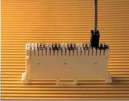
The QDF 2 and 4-wire test/patch cords provide access to circuits for testing, monitoring, and temporary or permanent patching.
