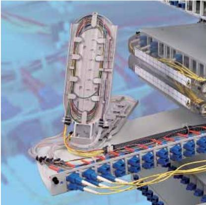
The front patching/splicing shelf, FOMS-FPS, is a multi-purpose mechanical shelf assembly for a fiber management system in a rack environment. Its compact design and high-density capacity allow the FOMS-FPS to deliver carrier-class fiber management to central offices, POPs, FTTx, mobile systems and LANs.
