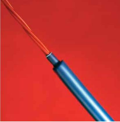
SCL is a semi-rigid heat-shrinkable tubing with a meltable inner wall, designed to provide one-step moisture-proof encapsulation to a wide variety of electrical parts including wire splices, breakouts and electronic components. When cooled, the entire mass becomes a rigid, tough, homogeneous covering with a controlled wall thickness.
