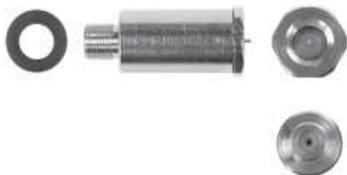
This high pass filter rejects the upstream frequency band. Its purpose is to block ingress from the subscriber side in case of unidirectional (downstream) signal distribution. Cable operators install it mostly at the output of taps.
