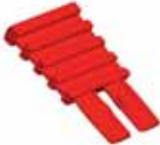
The dummy plug is a plastic device which denies access of test or break plugs to the circuit when inserted into the access slot of a UCS-DM & UCS-CM magazine. It can be used for marking special circuits and for preventing accidental interruption of designated lines.
