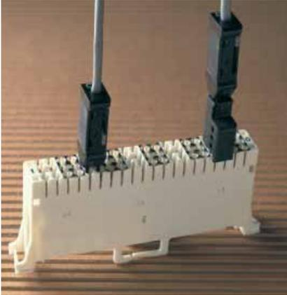
The 4-wire retractable test/patch cord consists of a plastic plug assembly containing a moulded printed circuit board which can be extended from or retracted into the housing assembly. This unique design enables access for testing or monitoring circuits on the QDF-E termination magazine both with or without installed protectors.
