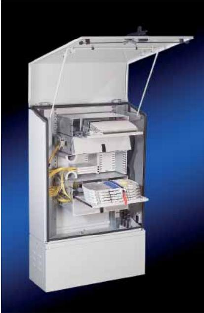
The FIST street cabinet, FIST-CAB5, is an all purpose metal outdoor cabinet designed to accommodate the FIST generic shelf family. It offers dust-proof, environmental and me-chanical protection for the fiber management functions of splicing, patching and passive component integration.
