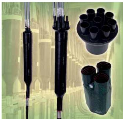
The VCKT closure system is used for distribution of telecommunication cables in telephone exchanges. A heat-shrinkable RayFort sleeve, used in conjunction with a metal canister and a multiple break-out part protects the splice.
