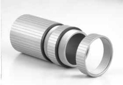
These female-to-male threaded connector are designed to secure inner ducts to cabinets and junction boxes. They consist of a universal threaded coupling end and a nipple end with locking washers and gaskets. The connectors attach to standard knockout sizes in panels and racking for maximum security to premises cabling, eliminating cable kink at these transitions.
