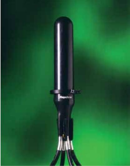
RABC is a fully sealed closure combining a mechanical dome with reliable heat-shrinkable sealing for the cables. It is suitable for use as an aerial or underground joint closure in both new construction and maintenance applications in the distribution network, typically in the rehabilitation of expanding plugs, tape and 31A type resin joints.
