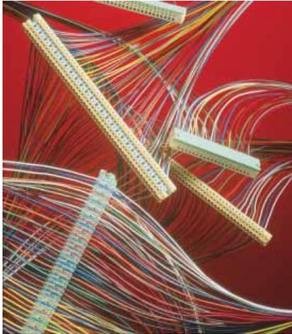
The AMP STACK MARK III 25 pair connectors are designed to mass terminate communication cables of solid copper or aluminum conductor wires ranging from 0.32 to 0.8 mm of diameter, (28 to 20 AWG).
