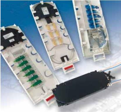
The coarse wavelength division multiplexing technique combines (or multiplexes) two or more signals with different wavelengths in one common fiber. The same components can also be used to separate the wavelengths (de-multiplexing) at the remote location. These devices are integrated into the Tyco Electronics FOSC range of fiber-optic splicing trays. This allows for easy integration in enclosures, wall-mount boxes, or ODFs.
