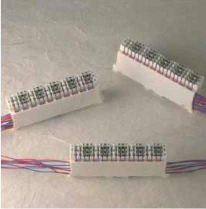
Wire guides for jumper wires are optionally available. These facilitate wire management by guiding the wires through access slots straight to their contact and finishing positions.
