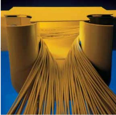
The LIGHTRAX fiber optic raceway system is a fully enclosed ducting system that segregates, routes and protects fiber optic cables and jumpers from building entry point to fiber termination and distribution equipment. With the raceway system, fiber is easily traced and accessed through its convenient fully wrap-around lay-in design. It also maintains complete separation from twisted pair and coax cable.
