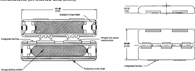
For splice protection and sheath repair\* of 2-pair drop wire telephone cable.
