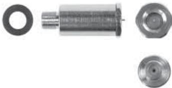
This high pass filter rejects the upstream frequency band. Its purpose is to block ingress from the subscriber side in case of unidirectional (downstream) signal distribution. Cable operators install it mostly at the output of taps.
