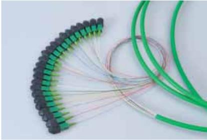
The Tyco Electronics Mini-Breakout cables are developed to be a very compact cabling solution for riser applications in MDU's. With the cable strength elements integrated in the individual fiber elements, Pico-Breakout, the cable becomes very small in diameter and very flexible to be pulled vertically through the riser.
