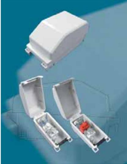
The subscriber connector unit is used for the connection of an outdoor to an indoor drop wire. It consists of a rectangular box base with a cover and a five-pole connection module secured to the base.
