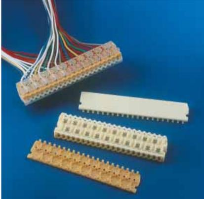
The AMP STACK MARK IV connector family is designed to mass terminate communication cables of solid copper or aluminum conductors ranging from 0.4 to 0.9 mm or diameter (26 to 19 AWG).
