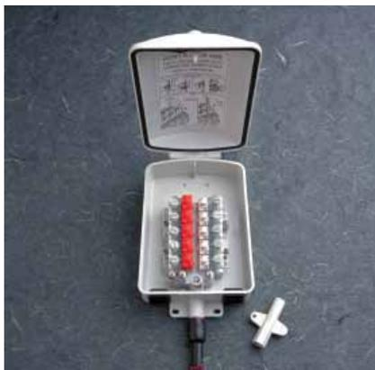
This is used in terminating cables of secondary telephone networks to the cable pairs of subscriber lines. It consists of a body and cover which house a VX stubbed block.
