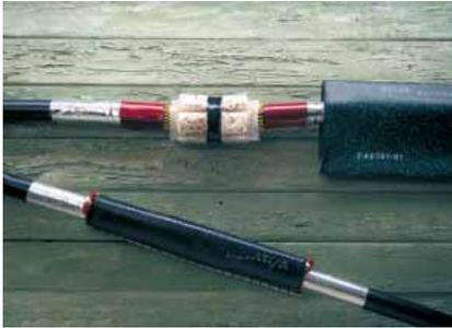
The ACBS product is a unique adhesive cable blocking system providing a water and pressure block for air-core cables up to 400 pairs. The system consists of heat-shrinkable thick-wall tubing (for new constructions) or RayFort wraparound sleeves (for maintenance) covered with thermo-indicating paint and pre-assembled bags containing a specific amount of specially developed adhesive granules.
