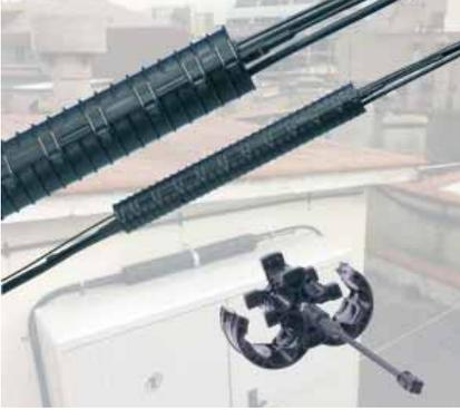
The TTRC closure has been developed for the environmental protection of aerial telecommunication joints up to 600 pairs. The product consists of two sealing units and a central body, which mechanically protects the joint.
