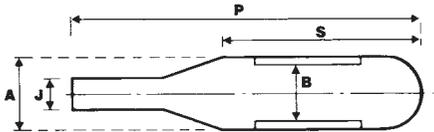
PEDCAP is a general purpose single-ended closure designed for a variety of applications in a distribution network. It is suitable for use as an aerial or underground joint closure in both new construction and maintenance applications, typically in the rehabilitation of tape and plug expanding joints.
