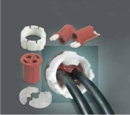
Tyco Electronics' Biplex plugs seal one or two cables in a (nominal) 50mm O.D. (with 4.6mm wall) duct.
