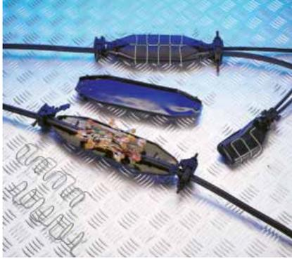
Three sizes of Gelsnap are available for the protection of paper/lead or plastic cable joints of up to 30 pairs. The product is quick to install and easy to use. No special tools are required. The use of non-flowing gel under permanent pressure prevents water ingress. It is robust and reliable under a wide variety of environmental conditions. Many connector types can be accommodated. Butt, in-line, and branch configurations are possible. Re-entry is easy and clean.
